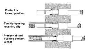
Insert Lock - the contact has a ridge (shoulder) machined around the contact which snaps into place in the spring clips (tines) located inside each cavity of the insert. The contacts are usually inserted from the rear of the connector and removed either from the front or rear of the connector.
