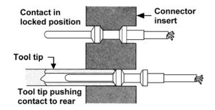
2. Contact Lock - the locking device is located on the contact itself in the form of a spring finger which snaps into place on a ring inside the insert. The contacts are usually inserted from the rear of the connector and removed from the front (face) of the connector.
